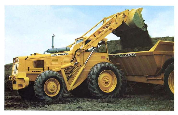
The LM 840 loads fast. This is due to excellent bucket filling, quick manoeuvring assisted by the tight turning radius, and simplified load distribution as a result of long reach.
