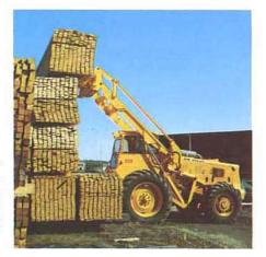
The LM 840 is well suited to the stacking of palletized goods and sawn timber, thanks to the combination of good reach and generous lifting height. The machine can stretch high over the growing stack, which provides a support when placing the final pallet or package.
