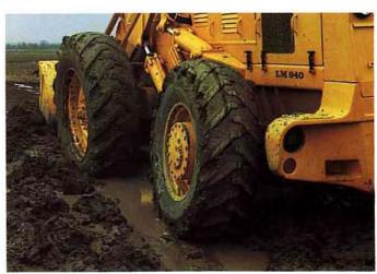
On loose or slippery surfaces the specific ground pressure and contact area are vital factors in the machine's ability to keep moving. The LM 840 fully satisfies these conditions and, despite its weight, can carry on in places where many machines would experience difficulty in working.
