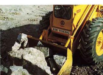
The remarkably high penetration force of the LM 840 assists effective bucket tilling. In combination with the large wheels and ideal weight distribution (= low ground pressure) and balanced transmission (= stepless torque multiplication, plus differential-lock feature) the result is a high-output machine that maintains performance even under adverse conditions.
