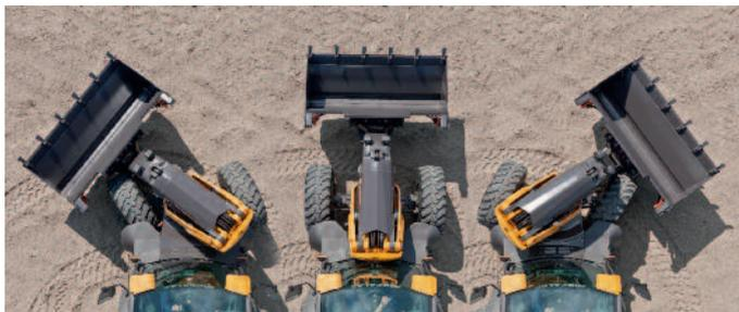
The slender monoboom increases the working area between the wheels by 32%
