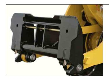
**Skid Steer Loader Coupler.** The universal skid steer loader coupler allows the use of many Cat Skid Steer Loader work tools. Using either the standard or high flow hydraulic option, this coupler allows the H-Series Compact Wheel Loaders to integrate into a skid steer loader fleet.
