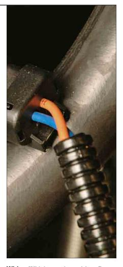
Wiring. With heavy-duty wiring, Cat Compact Wheel Loaders offer great electrical durability. The water resistant sealed connectors prevent dust and moisture interfering with the electrics. Multicoloured wiring is used to ease diagnosis and fault finding.
