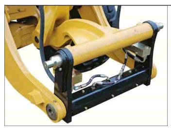
**Horizontal Pin Coupler.** This quick coupler will pick up the new range of Compact Wheel Loader work tools. The coupler along with the profiled loader arms have been designed to give maximum visibility to the work tool.
