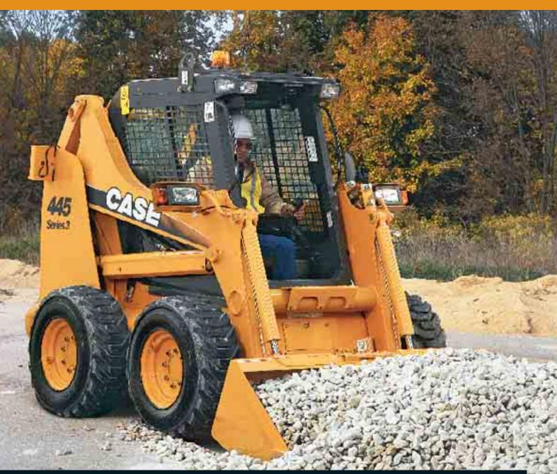
Operating load Engine Horsepower Operating weight **410 Series 3** 680 kg 45 kW - 60 hp 2463 kg **420 Series 3** 839 kg 55 kW - 74 hp 2996 kg **430 Series 3** 907 kg 61 kW - 82 hp 3084 kg **435 Series 3** 998 kg 61 kW - 82 hp 3075 kg **440 Series 3** 998 kg 67 kW - 90 hp 3193 kg **445 Series 3** 1134 kg 61 kW - 82 hp 3683 kg
