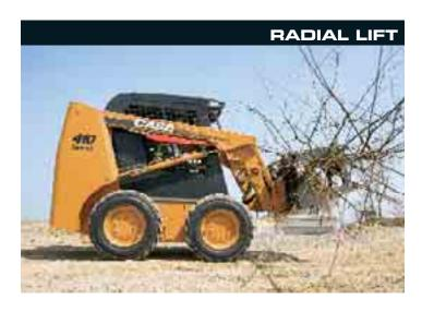
On 410, 420, 430, 440 series 3 the kinematics is of the radial type. This means that he arm is articulated at its base by a single pin. This conception is the most common in the market. Its robustness combined with the arms being in contact with the chassis in its low position make these models even more accurate for all demanding digging applications. Loading/unloading can be made easier by ordering the self - level (raise) option.
