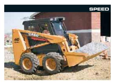
Productivity on 420, 430, 440 series 3 is vastly improved by blazing two-speed travel of 17 to 18 km/h. 410 with one speed only reaches 10 km/h.
