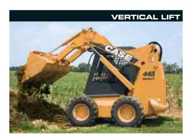
On 435, 445 series 3 the kinematics is of the vertical type. This means that the arm is articulated at its base by a heavy lift and reach linkage which makes loading/unloading in elevation easier. As for the radial lift units, the arm is in contact with the chassis in its low position giving these models good digging abilities as well.
