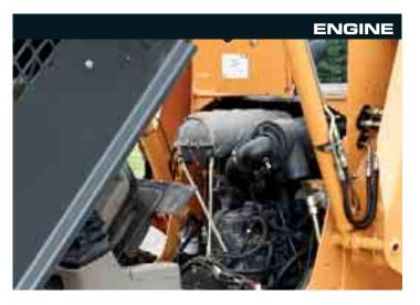
The Case Series 3 skid steers are all powered by Turbo, 4 cylinder, tier 3 emission certified, diesel engines designed for Case with efficiency and fuel economy in mind.
