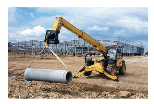
**Quick Coupler.** An IT interface is standard on the B-Series. It is available in both a manual and a hydraulic version.
