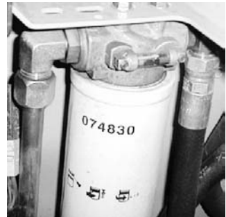
Figure 40 Hydraulic Oil Filter and Indicator
